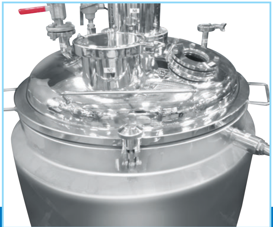
Close view of Binder Vessel Lid
