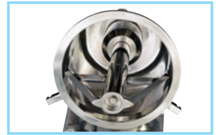
Sanitary Process Chamber Design
