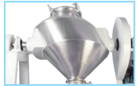
Asymmetric Double Cone Design
