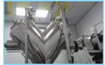
'V' Design for Diffusion Blending
