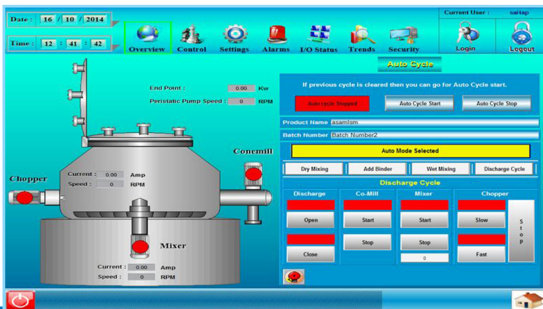
Mimic Display for Process Monitoring and Control
