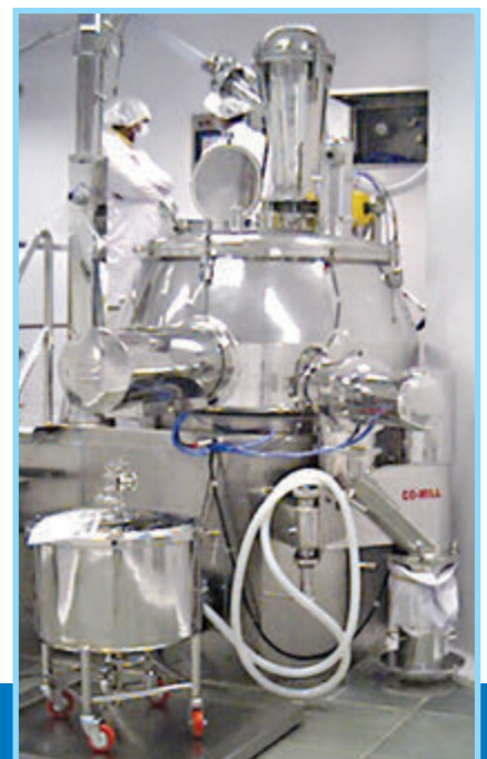
Product charging through closed loop vacuum transfer
