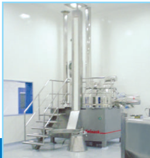
Product charging through gravity transfer
