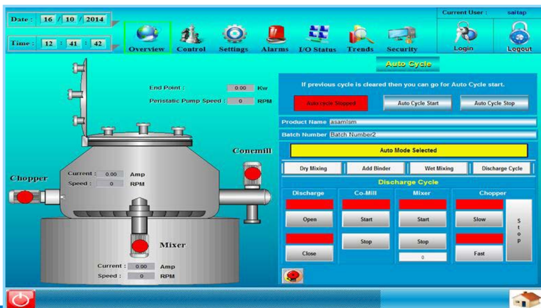
Mimic Display for Process Monitoring and Control
