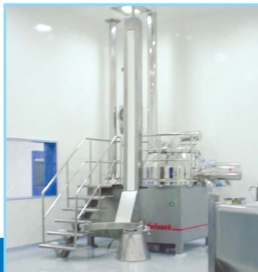
Product charging through gravity transfer
