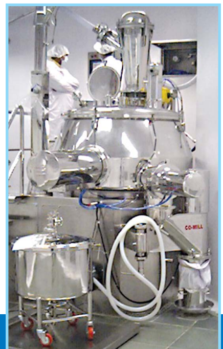
Product charging through closed loop vacuum transfer
